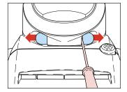
When the end caps are removed, the hinging pin can be removed and the hinge can be taken off the appliance.
